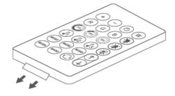
Make sure the IR remote aims at the IR receiver within the sensing distance. The angle of the IR receiver is 120 and the sensing distance is 5 meters. Please remotely control within the sensing range.
