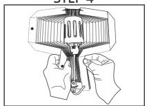
FIX THE SOCKET IN THE CENTER OF THE SHADE BY PLACING THE HOOK ON ELECTRICAL WIRE .
